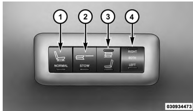
Rear Panel Power Switch Bank
