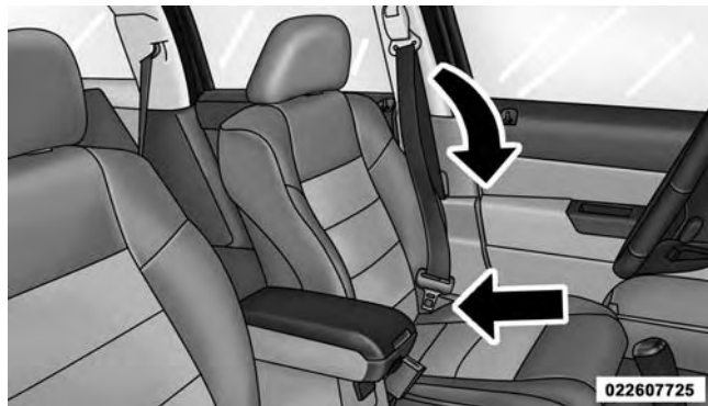
Inserting Latch Plate Into Buckle
