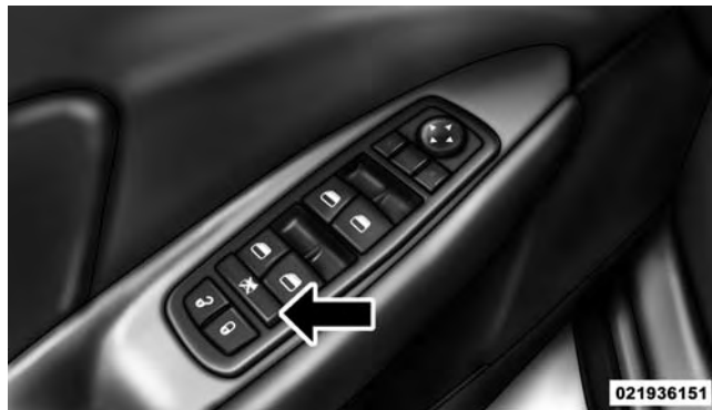
Window Lockout Switch
