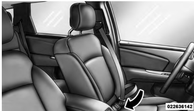
Connecting Latch Plate To Buckle
