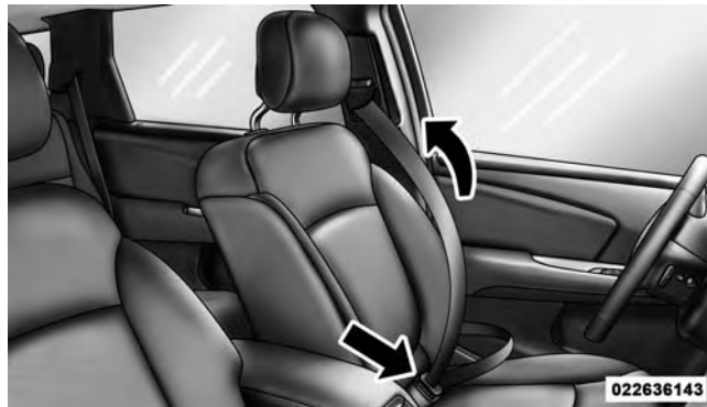
Removing Slack From Belt
