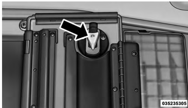
Storage Bin Cover Emergency Release Lever
