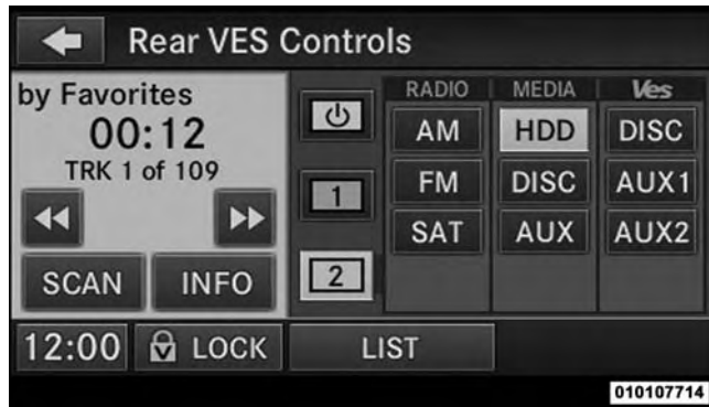
Select Channel/Screen 2 And HDD In The Media Column
