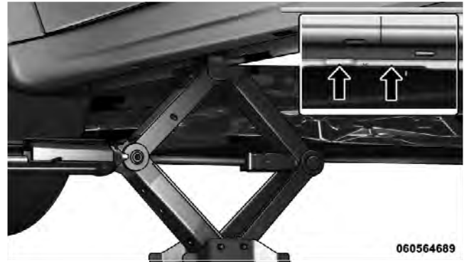
Front Jacking Location
