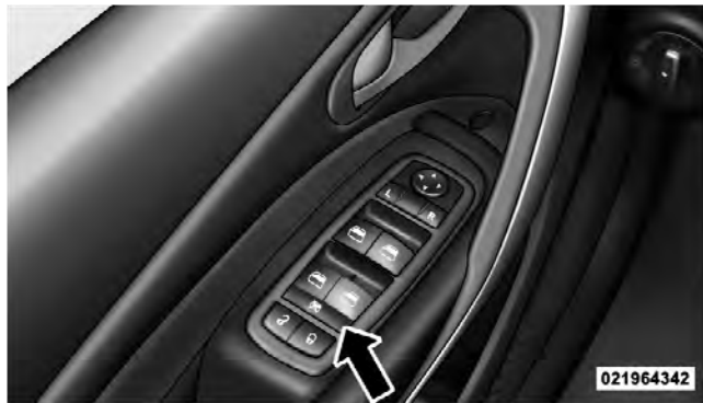
Window Lockout Switch
