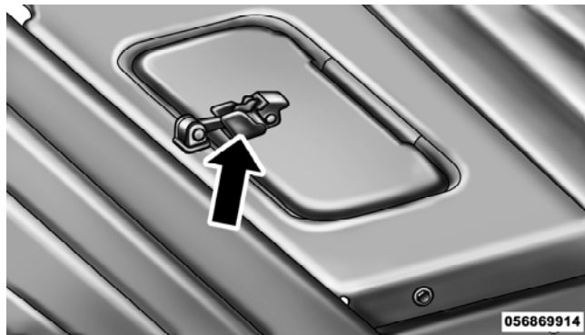
Manual Shut Off Valve Access Door
