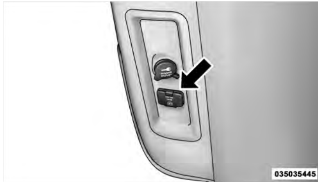
Power Inverter Outlet
