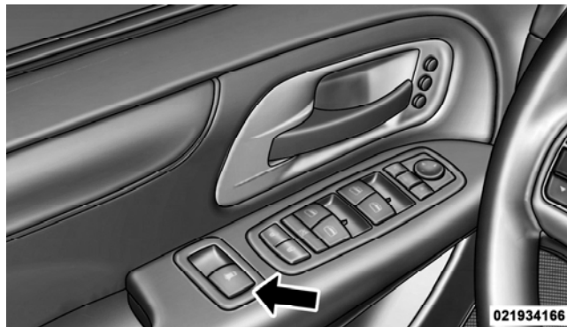
Power Vent Window Switch Open/Close
