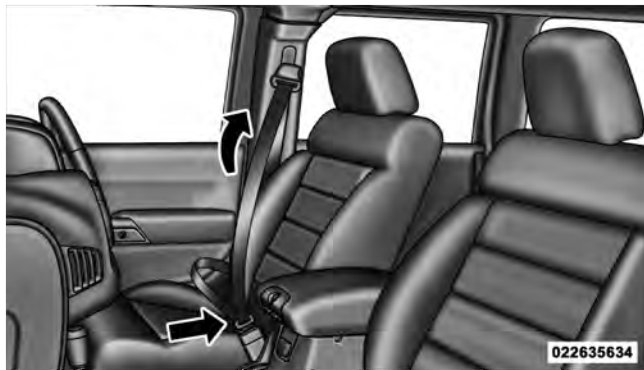
Removing Slack From Belt
