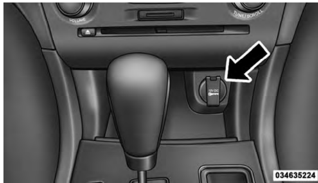
Front Power Outlet
