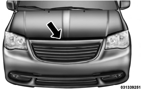
Safety Catch Location
