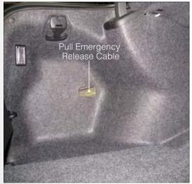
• To manually open the fuel door, remove the cover and pull the release cable located in the trunk.
