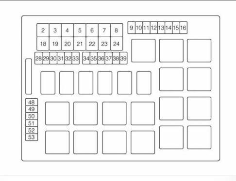
• The Integrated Power Module (fuses) is located in the engine compartment on the right hand side near the Washer Fluid Reservoir. This module contains fuses and relays.
