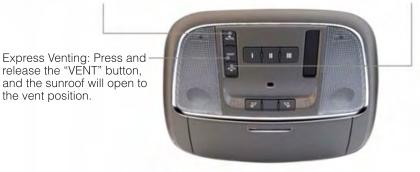
The power sunroof switches are located on the overhead console.
