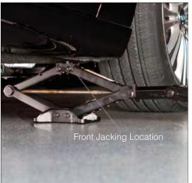
5. Raise the vehicle just enough to remove the flat tire and install the spare tire.
