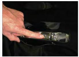
Both front door handles have LOCK buttons located on the outside of the handle. With one of the vehicle's Keyless Enter-N-Go Key Fobs located outside the vehicle and within 5 ft (1.5m) of the driver's or passenger front door handle, press the door handle LOCK button to lock all four doors and trunk.
