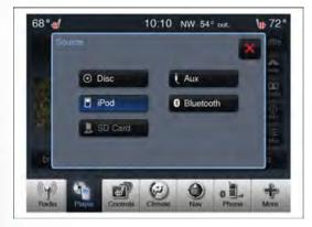
The iPod<sup>®</sup>/CD/AUX controls are accessed by touching the Player soft-key to enter the Player main screen, then touch the source soft-key and choose between Disc, AUX, iPod<sup>®</sup>, Bluetooth or SD Card.
