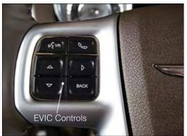
the UP  $\triangle$  or DOWN  $\nabla$  button until System Setup displays, then press the SELECT  $\triangleright$  button. Scroll through the settings using the UP or DOWN buttons. Press the SELECT  $\triangleright$  button to change the setting. Press the BACK button to scroll back to a previous menu or sub menu.
