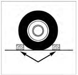
Block the front and rear of the wheel diagonally opposite of the jacking position. For example, if changing the right front tire, block the left rear wheel.
