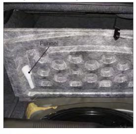
A funnel is provided (located in the trunk in the spare tire area) to open the flapper door to allow for emergency refueling with a gas can.
