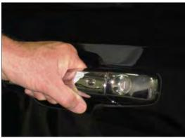
With a valid Keyless Enter-N-Go Key Fob located outside the vehicle and within 5 ft (1.5m) of the driver or passenger side door handle, grab either front door handle to unlock the door automatically.
