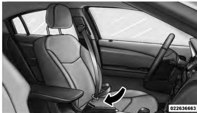
Inserting Latch Plate Into Buckle
