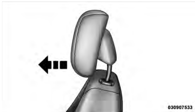
Active Head Restraint (Tilted)
