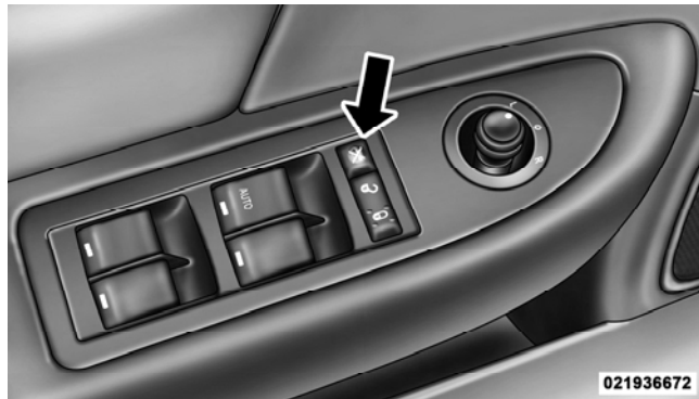
Window Lockout Switch
