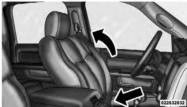
Removing Slack From Belt
