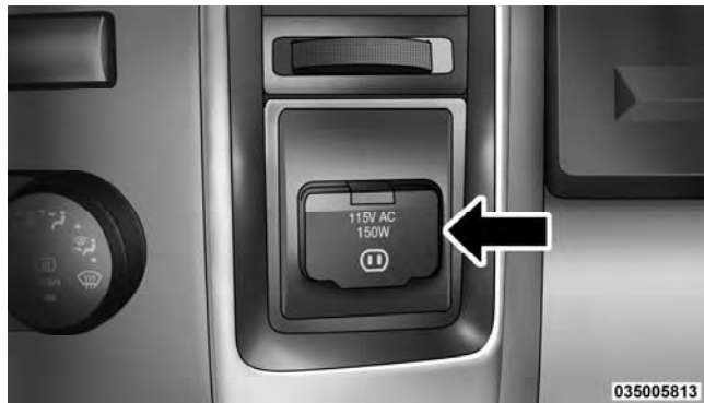
Power Inverter Outlet
