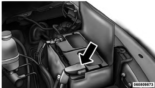
Positive Battery Post
