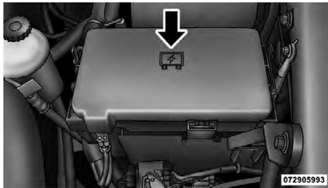
Totally Integrated Power Module
