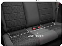
Loosen the child seat adjusters on the lower straps and tether straps so that you can attach the hook or connector to the lower and tether anchorages more easily.
