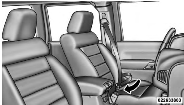
Inserting Latch Plate Into Buckle
