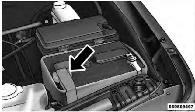
Positive Battery Post
