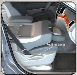
The front passenger seat can be folded flat to allow for extended cargo space. Pull up on the recliner lever to fold down the seatback.
