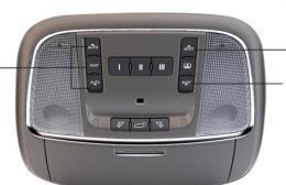
Express Close Power Shade: Press the switch forward and release. The shade will close automatically from any position.
