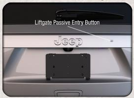
With a valid Keyless Enter-N-Go Key Fob within 3 ft (1.0m) of the liftgate, press the button located to the right of the liftgate handle to unlock the liftgate. Press the button a second time to lock the liftgate.
