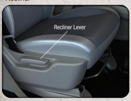
Lift the rear lever located on the outboard side of the seat, lean back and release when seat is in desired position.
