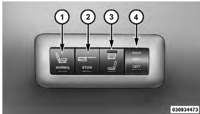
Rear Panel Power Switch Bank
