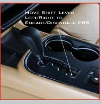
Electronic Range Select (ERS) allows you to limit the highest available transmission gear, and can be activated during any driving condition. When towing a trailer, using ERS shift control will help you maximize both performance and engine braking.
