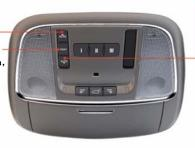
THE POWER SUNROOF SWITCHES ARE LOCATED ON THE OVERHEAD CONSOLE.
