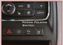
For improved visibility, the third row head restraints can be folded using a switch, located on the instrument panels switch bank.
