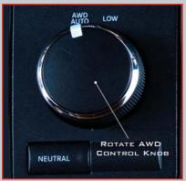
This is an electronic shift transfer case and is operated by the AWD Control Switch (Transfer Case Switch), which is located on the center console.
