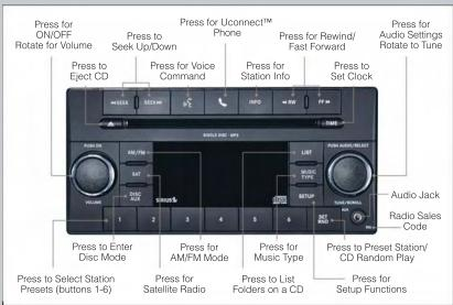
**NOTE:** Your radio may not be equipped with the Uconnect™ Voice Command and Uconnect™ Phone features. To determine if your radio has these features, press the Voice Command button on the radio. You will hear a voice prompt if you have the feature, or see a message on the radio stating "Uconnect Phone not available" if you do not.
