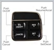
The speed control switches are located on the steering wheel.
