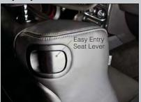
Pull forward on the lever, located on the side of the seatback, to dump the seatback forward and slide the seat forward. You can also temporarily remove the seat belt from the guide loop on the seat and allow the seat belt to retract out of the way. This allows for easier access to the rear seat.
