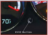
The EVIC features a driver interactive display that is located in the instrument cluster. For additional information, refer to Programmable Features in this guide.
