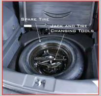
• The jack and jack-handle are stowed under the load floor in the trunk.
