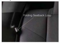
To fold the rear seatback forward, pull on the loops to fold down either or both seatbacks.
