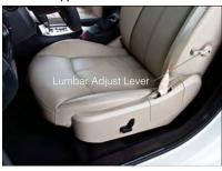
The lumbar adjust lever is on the outboard side of the seatback. Rotate the lumbar adjust lever downward to increase the lumbar support or upward to decrease the lumbar support as desired.
