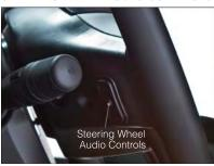
The steering wheel audio controls are located on the rear surface of the steering wheel.
