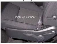
The height adjustment control lever is located on the outboard side of the seat. Raise the lever to raise the seat. Lower the lever to lower the seat.
