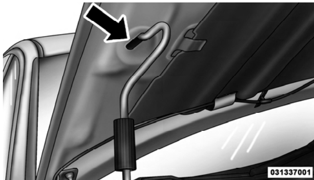
Hood Prop Rod Hole Location
