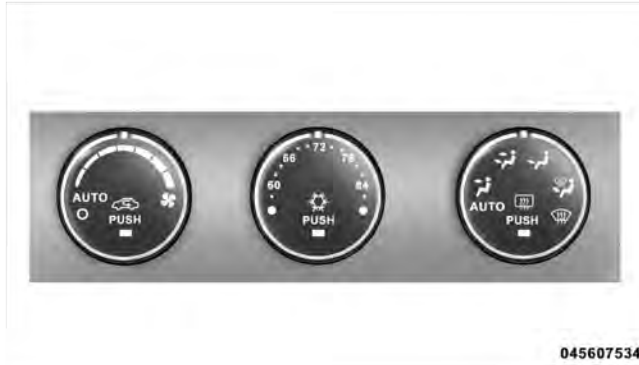
Automatic Temperature Control
