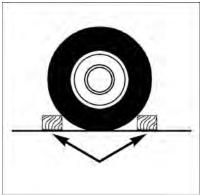
Block both the front and rear of the wheel diagonally opposite of the jacking position.
