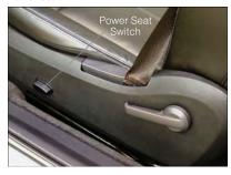
The power seat switch, located on the outboard side of the seat near the floor, controls forward/back, up/down, and tilt adjustment.
