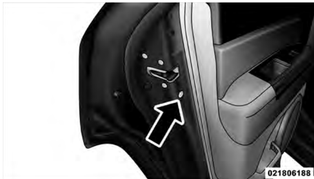
Child-Protection Door Lock Location
