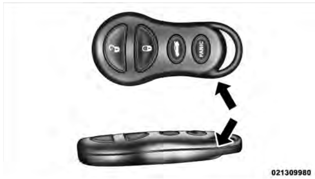
Separating RKE transmitter Halves
