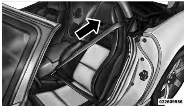
Removing Slack From Belt (Convertible Shown)
