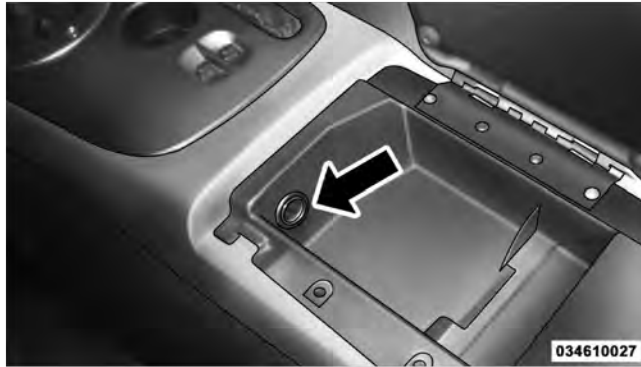
Center Console Power Outlet
