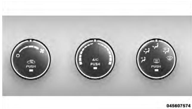
Manual Temperature Control
