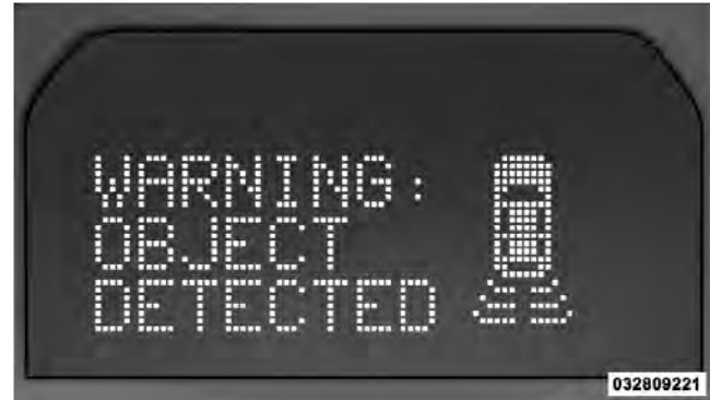
ParkSense® Warning Display
