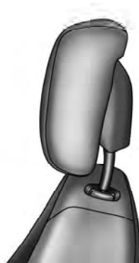
Active Head Restraint (Normal Position)
