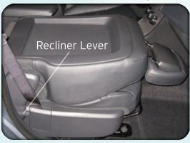
The front passenger seat can be folded flat. Pull up on the recliner lever to fold down the seat back.
