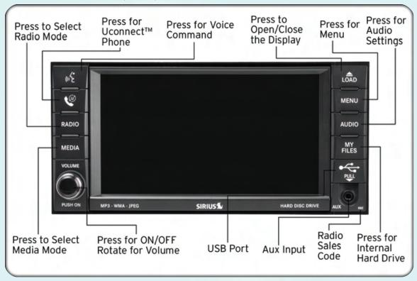
**NOTE:** Uconnect<sup> $\top$ M</sup> Phone and Voice Command are vehicle options which must be ordered separately. The buttons on the radio will only be active if the vehicle has been equipped with the option.
