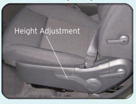
The height adjustment control lever is located on the outboard side of the seat.
