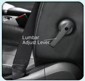
The lumbar adjust lever is on the outboard side of the seatback. Rotate the lumbar adjust lever downward to increase the lumbar support or upward to decrease the lumbar support as desired.
