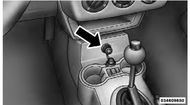
Front Power Outlet
