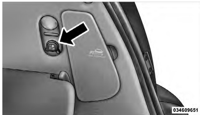
Rear Power Outlet
