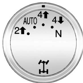
Two Speed Transfer Case
