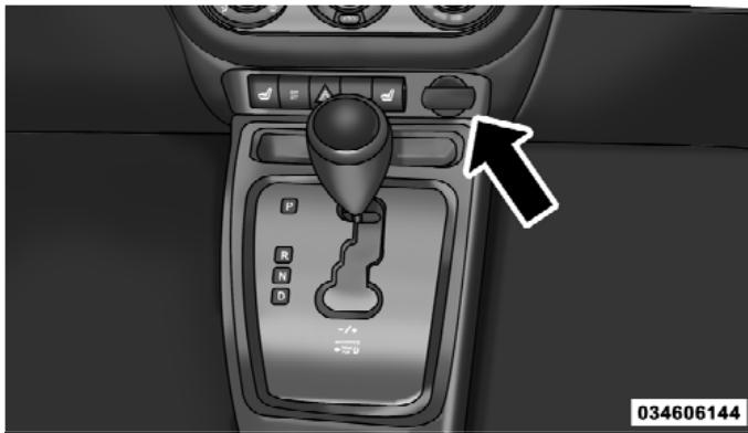
Power Outlet 12-Volts
