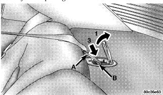
2. Route the tether strap to provide the most direct path for the strap between the anchor and the child seat. If your vehicle is equipped with adjustable rear head restraints, raise the head restraint and, where possible, route the tether strap under the head restraint and between the two posts. If not possible, lower the head restraint and pass the tether strap around the outboard side of the head restraint.
