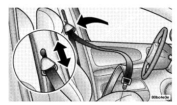
As a guide, if you are shorter than average, you will prefer a lower position, and if you are taller than average, you'll prefer a higher position. When you release the anchorage, try to move it up or down to make sure that it is locked in position.
