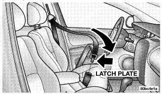
3. When the belt is long enough to fit, insert the latch plate into the buckle until you hear a "click."
