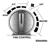
Use this control to regulate the amount of air forced through the system in any mode you select. The fan speeds to the left of the OFF position are for Air Conditioning. Choosing one of these speeds turns on the air conditioning compressor. The
