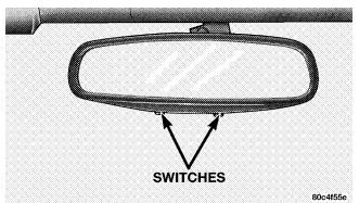
**NOTE:** The map lights will remain on when the ignition switch is in the Run or Accessory positions.
