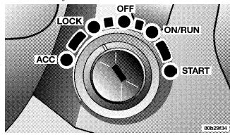
**NOTE:** If you try to remove the key before you place the lever in PARK, the key may become trapped temporarily in the key cylinder. If this occurs, rotate the key clockwise slightly, then remove the key as described. If a malfunction occurs, the system will trap the key in the ignition cylinder to warn you that this safety feature is
