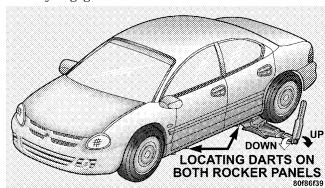
4. Raise the vehicle by turning the jack screw to the right. Raise the vehicle only until the tire clears the surface. Miminum tire lift provides maximum vehicle stability.
