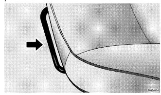
Using body pressure, move forward and rearward on the seat to be sure the seat adjusters have latched after the adjustment bar is released.
