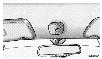
A single control "tilts" the sunroof to the vent position and also slides the sunroof rearward to the full open position. Move the switch rearward to move the sunroof panel to the full vent position. The sunroof can be stopped at any position between closed and full vent open.
