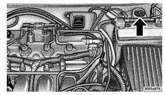
Use only manufacturers recommended brake fluid, refer to Recommended Fluids, Lubricants and Genuine Parts for correct fluid type.
