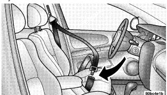
2. The seat belt latch plate is above the back of the front seat, next to your arm in the rear seat. Grasp the latch plate and pull out the belt. Slide the latch plate up the webbing as far as necessary to allow the belt to go around your lap.
