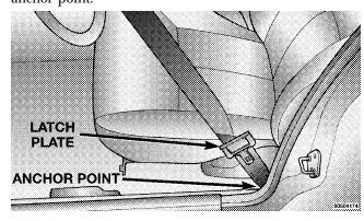
2. At about 6 to 12 inches above the latch plate, grasp and twist the belt webbing 180° to create a fold that begins immediately above the latch plate.
