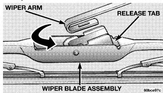
4. Install the new blade assembly onto the wiper arm tip until it locks in place.
