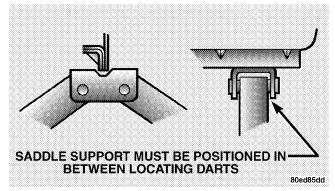
Do not raise the vehicle until you are sure the jack is securely engaged.
