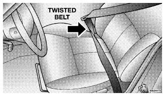
1. Position the latch plate as close as possible to the anchor point.
