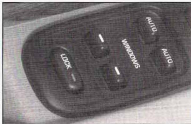
The power window controls located on the driver's door armrest operate each of the windows while the ignition is on or while Retained Accessory Power (RAP) is active. In addition, each passenger door has a control for its own window. See "Retained Accessory Power (RAP)" under *Ignition Positions* on page 2-22 for more information.
