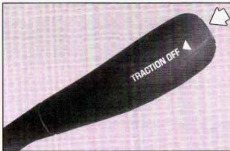
To turn the system off, press the TRACTION OFF button located at the end of the shift lever on the right side of the steering wheel.
