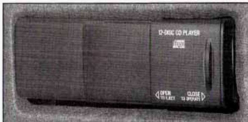
With the optional compact disc changer, you can play up to 12 discs continuously. Normal size discs may be played using the trays supplied in the magazine.
