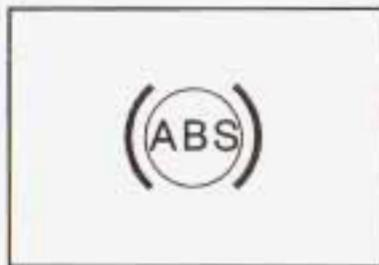
If there's a problem with the anti-lock brake system, this warning light will stay on. See *Anti-Lock Brake System Warning Light* on page 3-39.
