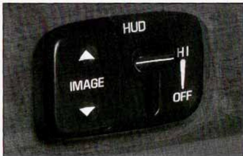
The HUD controls are located on the instrument panel to the left of the steering wheel.
