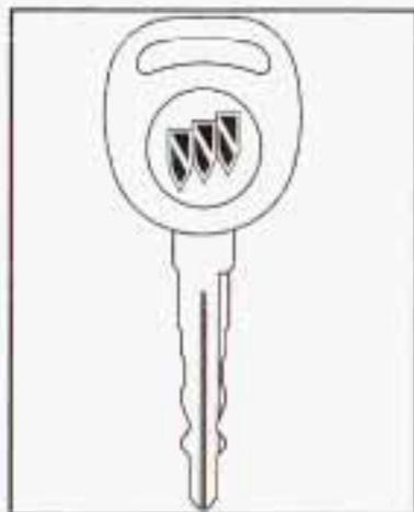
There is a master key that works in all of the lock cylinders (driver's door, trunk, ignition, and glove box).
