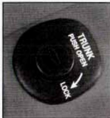
The TRUNK release button is located on the driver's door trim map pocket.
