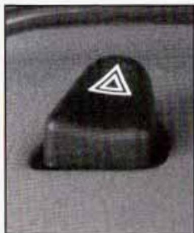
The hazard warning flasher button is located on top of the steering column.
