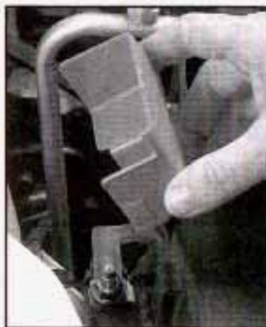
5. Access the remote positive (+) terminal by removing the cover.
