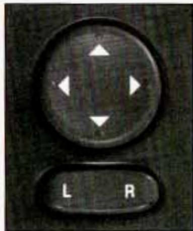
The controls for the outside power mirrors are located on the driver's door armrest.
