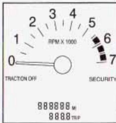
If your vehicle has this feature, the tachometer tells you how fast the engine is running. It displays engine speed in thousands of revolutions per minute (rpm).
