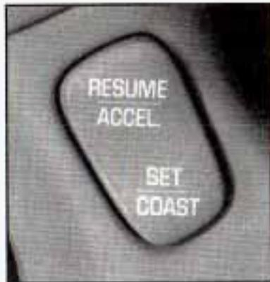
The switches to operate cruise control are located on the steering wheel.
