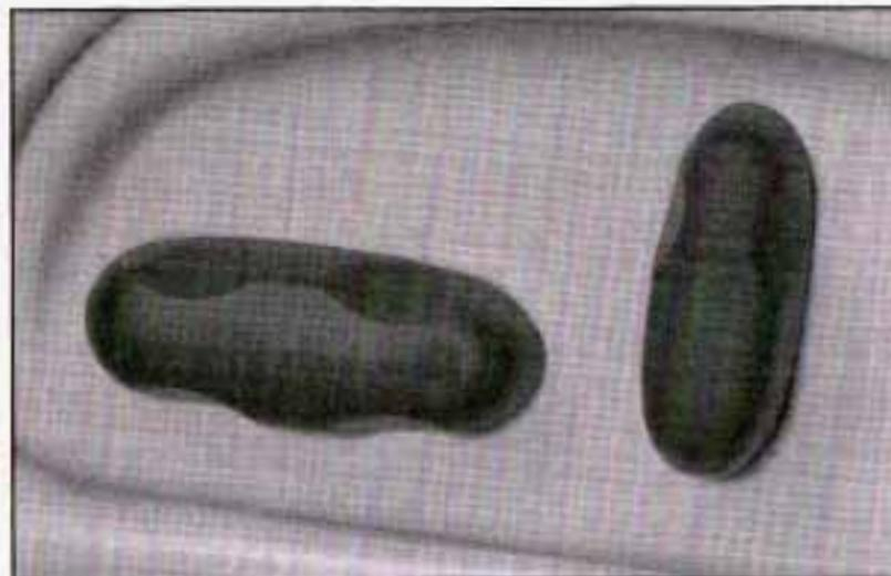
If your vehicle has this feature, the controls for the power seats are located on the outboard side of each front seat.
