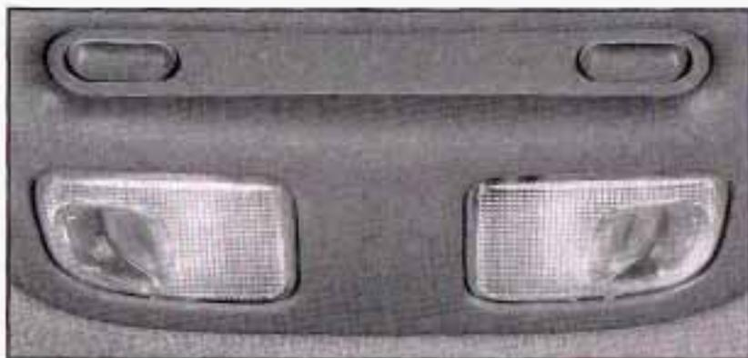
The front reading lamps, located on the headliner, are turned on or off by pressing one of the buttons located near each lamp.
