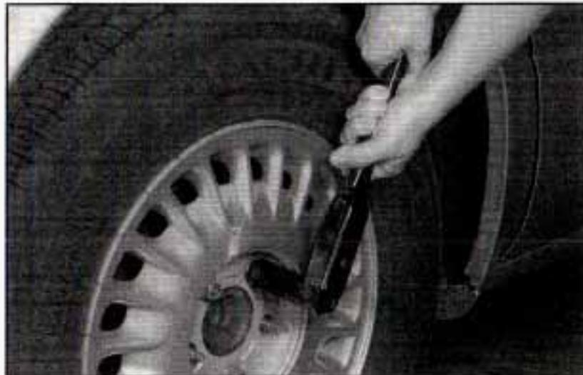
1. Use the wheel wrench to loosen the wheel nuts, but don't remove them yet.
