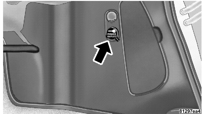
Rear Power Outlet
