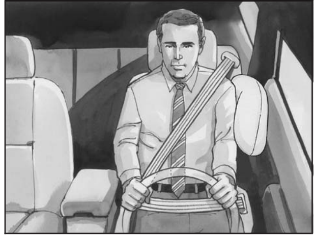
The driver's side impact air bag is in the side of the driver's seatback closest to the door.
