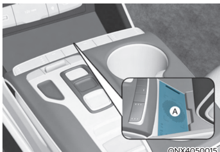
[A] : Wireless Charging Pad (In-vehicle Authentication Pad)
