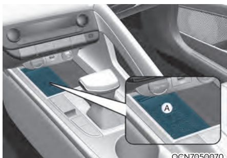
[A] : Charging pad
