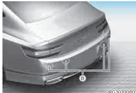
[A]: Rear view camera, [B]: Rear ultrasonic sensors
