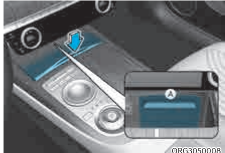
[A] : In-vehicle authentication pad (Wireless charging pad)
