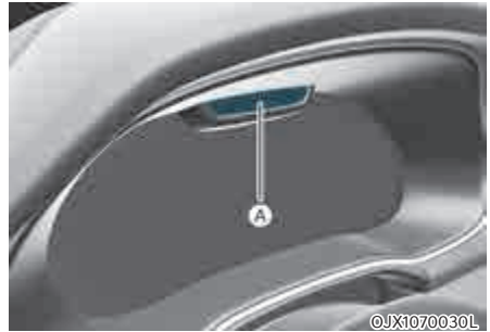
[A] : Interior view camera
