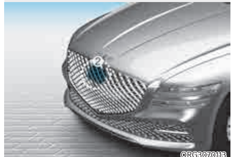
[1]: Front view camera, [2]: Front radar
