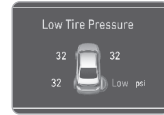
Low Tire Pressure Position Telltale and Tire Pressure Telltale (Shown on the LCD display)
