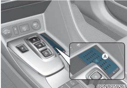
[A] : Wireless Charging Pad (In-vehicle Authentication Pad)
