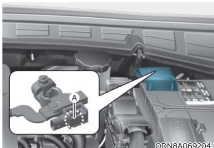
[A] : Battery sensor
