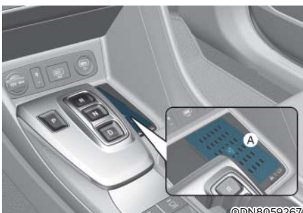
[A] : Wireless Charging Pad (In-vehicle Authentication Pad)
