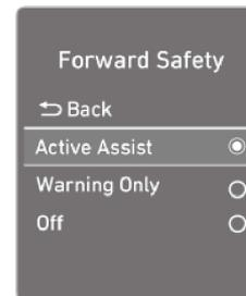
The Forward Collision Avoidance (FCA) system is designed to detect and monitor the vehicle ahead and warn the driver if a collision is imminent. This feature also allows pedestrian detection.
