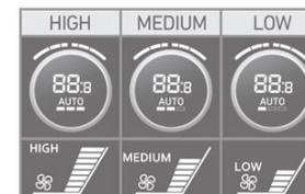
1. The fan speed is controlled automatically in 3 available settings.
