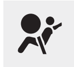
SRS warning light
