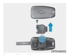
Battery Type: CR2032 To replace the battery:
