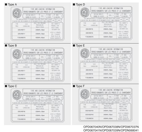
The label located on the driver's door sill gives the original tire size, cold tire pressures recommended for your vehicle, the number of people that can be in your vehicle and vehicle capacity weight.
