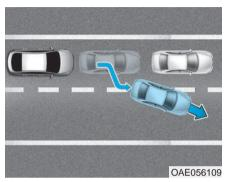
When driving in stop-and-go traffic, and a stopped vehicle in front of you merges out of the lane, the Forward Collision-Avoidance Assist system may not immediately detect the new vehicle that is now in front of you. In this case, you must maintain a safe braking distance, and if necessary, depress the brake pedal to reduce your driving speed in order to maintain a safe distance.
