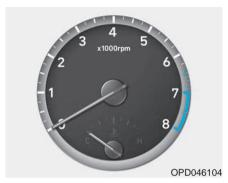
The tachometer indicates the approximate number of engine revolutions per minute (rpm).
