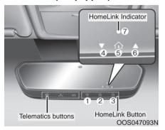
Your vehicle may be equipped with a Gentex Automatic-Dimming Mirror with a Z-Nav<sup>™</sup> Electronic Compass Display and an Integrated HomeLink<sup>®</sup> Wireless Control System. During nighttime driving, this feature will automatically detect and reduce rearview mirror glare while the compass indicates the direction the vehicle is traveling. The HomeLink<sup>®</sup> Universal Transceiver allows you to activate your garage door(s), electric gate, home lighting, etc.
