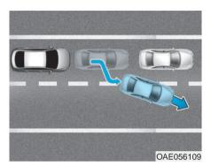
When driving in stop-and-go traffic, and a stopped vehicle in front of you merges out of the lane, the system may not immediately detect the new vehicle that is now in front of you. In this case, you must maintain a safe braking distance, and if necessary, depress the brake pedal to reduce your driving speed in order to maintain a safe distance.
