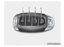
Your HYUNDAI uses a Smart Key, which you can use to lock or unlock a door (and liftgate) and start the engine.
