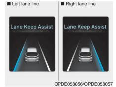
A visual warning appears on the cluster LCD display. Either the left lane line or the right lane line in the cluster LCD display will blink depending on which direction the vehicle is veering.
