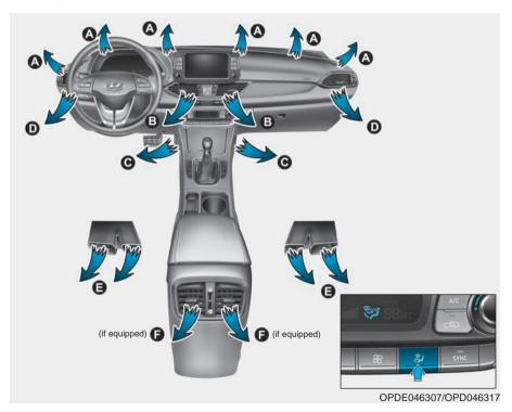
The mode selection button controls the direction of the air flow through the ventilation system.
