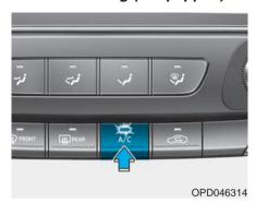
Push the A/C button to turn the system on (indicator light will illuminate) and off.
