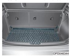
To keep items from shifting in the luggage compartment, you can use the 4 holders located in the luggage compartment to attach the luggage net.
