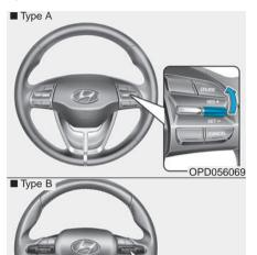
Push the toggle switch up (RES+) and hold it, while monitoring the SET speed on the instrument cluster.
