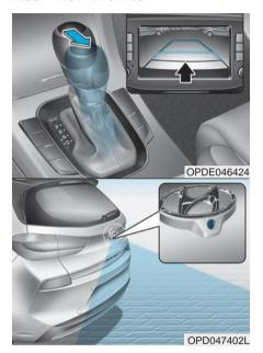
The Rear View Monitor will activate when the engine is running and the shift lever is in the R (Reverse) position.
