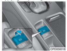
To apply the EPB (Electronic Parking Brake):
