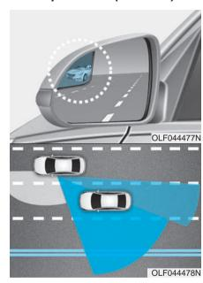
The Blind Spot Mirror (BSM) is a supplemental mirror that helps reduce the driver's blind spot by showing the rear side area of the vehicle. The blind spot mirror is equipped on the left-hand side view mirror.
