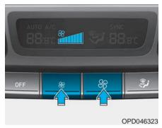
The fan speed can be set as desired by pushing the fan speed control button.
