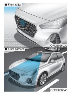
In order for the FCA system to operate properly, always make sure the sensor cover or sensor is clean and free of dirt, snow, and debris. Dirt, snow, or foreign substances on the sensor cover or sensor may adversely affect the sensing performance of the sensor.
