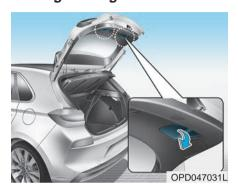
Lower the liftgate lid and press down until it locks. To be sure the liftgate lid is securely fastened, always check by trying to pull it up again without pressing the liftgate handle button.
