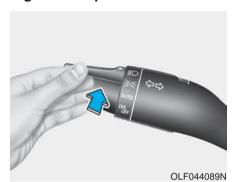
To turn on the high beam headlamp, push the lever away from you. The lever will return to its original position. The high beam indicator will light when the headlamp high beams are
