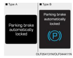
Parking brake automatically locked When the EPB is applied from Auto Hold, a warning will sound and a message will appear.
