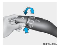
The High Beam Assist (HBA) is a system that automatically adjusts the headlamp range (switches between high beam and low beam) according to the brightness of other vehicles and road conditions.
