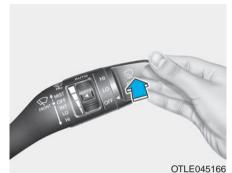
Push the lever away from you to spray rear washer fluid and to run the rear wipers 1~3 cycles. The spray and wiper operation will continue until you release the lever.
