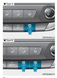
This button is used to select the outside (fresh) air position or recirculated air position.
