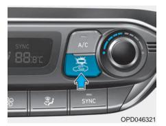
This button is used to select the outside (fresh) air position or recirculated air position.
