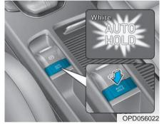
1. With the driver's door, engine hood and liftgate closed, fasten the driver's seat belt or depress the brake pedal and then press the [AUTO HOLD] switch. The white AUTO HOLD indicator will come on and the system will be in the standby position.
