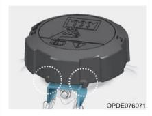
Make sure that the tiny protrusions inside the coolant cap is securely interlocked.
