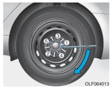
13. Use the wheel lug nut wrench to tighten the lug nuts in the order shown. Double-check each lug nut until they are tight. After changing tires, have an authorized HYUNDAI dealer tighten the lug nuts to their proper torque as soon as possible. The wheel lug nut should be tightened to 79~94 lbf-ft (11~13 kgf-m).
