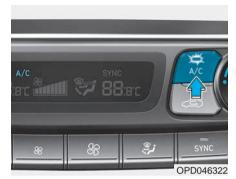
Push the A/C button to manually turn the system on (indicator light will illuminate) and off.
