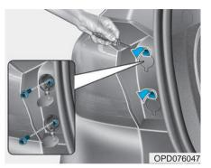
Stop/Tail lamp (Type A) and turn signal lamp
