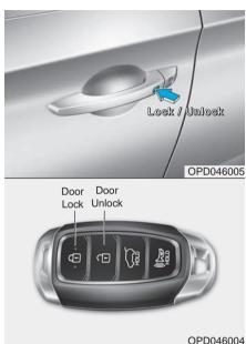
Press the button on the driver's outside door handle while carrying the Smart Key with you or press the Door Unlock button on the Smart Key, the driver's door will unlock. If you press the button on the front passenger's outside door, all doors will unlock.
