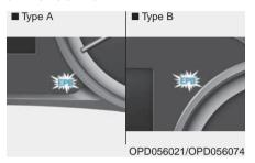
This warning light illuminates if the Engine Start/Stop button is changed to the ON position and goes off in approximately 3 seconds if the system is operating normally.
