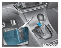
To open the cover, push the lip of the cover forward then release. The cover will open slowly. To close the cover, push the lip down to the closed position.
