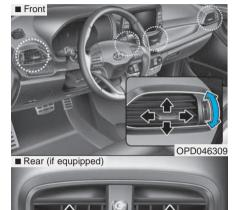
The outlet vents can be opened (⊜) or closed (○) separately using the thumbwheel.
