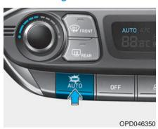
The Automatic Climate Control System is controlled by setting the desired temperature.
