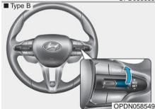
Push the toggle switch up (RES+). If the vehicle speed is over 20 mph (30 km/h), the vehicle will resume the preset speed.
