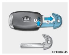
Move the release lever in the direction of the arrow (1) and then remove the mechanical key (2). Insert the mechanical key into the key hole on the door.
