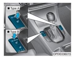
While the engine is running, push either of the switches to warm the driver's seat or front passenger's seat.
