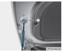
4. Pull out the support rod and hold the hood open with the support rod (1).
