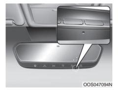
The Compass can be turned ON and OFF, but it returns to ON after the ignition is cycled.
