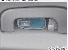
Your vehicle is equipped with LED lamps. LED lamps do not have replaceable bulbs. If the LED lamp does not operate, have the vehicle checked by an authorized HYUNDAI dealer.
