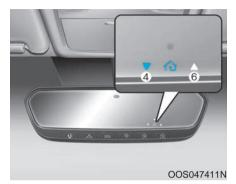
5. If both indicator (4) and (6) are flashing rapidly for about 5 seconds, the two way synchronization is completed.
