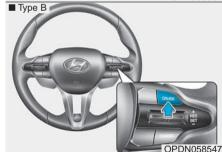
Push the CRUISE button on the steering wheel to turn the system on. The cruise ( C) CRUISE) indicator will illuminate.
