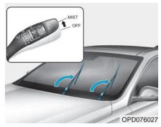
This vehicle has a "hidden" wiper design which means that the wipers cannot be lifted when they are in their bottom resting position.
