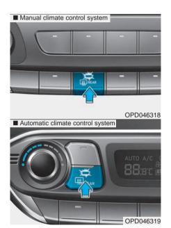
The defroster heats the window to remove frost, fog and thin ice from the interior and exterior of the rear window, while the engine is running.
