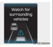
If the vehicle ahead (vehicle speed: less than 20 mph (30 km/h)) disappears to the next lane, the warning chime will sound and a message "Watch for surrounding vehicles" will appear. Adjust your vehicle speed for vehicles or objects that can suddenly appear in front of you by depressing the brake pedal.
