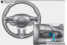
Push the toggle switch down (SET-) and hold it. Your vehicle will gradually slow down. Release the toggle switch at the speed you want to maintain.
