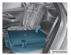
5. To use the rear seat, lift and unfold the seatback to the upright position. Push the seatback firmly until it clicks into place. Make sure the seatback is locked in place.
