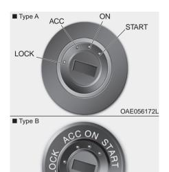
Whenever the front door is opened, the ignition switch will illuminate, provided the ignition switch is not in the ON position. The light will go off immediately when the ignition switch is turned on or go off after about 30 seconds when the door is closed. (if equipped)
