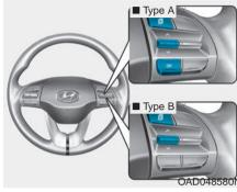
To change the trip mode, toggle the UP/DOWN arrow switch "  $\land$  ,  $\checkmark$  " on the steering wheel.
