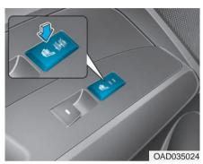
While the engine is running, push either of the switches to warm the rear seat.
