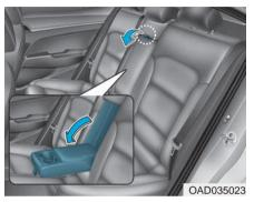
The armrest is located in the center of the rear seat. Pull the armrest down by using the strap from the seatback to use it.
