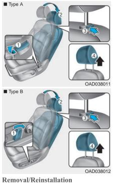
To remove the head restraint:
