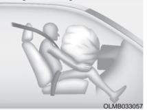
After complete inflation, the air bag immediately starts deflating, enabling the driver to maintain forward visibility and the ability to steer or operate other controls.
