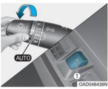
AUTO light position (if equipped) The parking lamp and headlamp will be turned ON or OFF automatically depending on the amount of light outside the vehicle.
