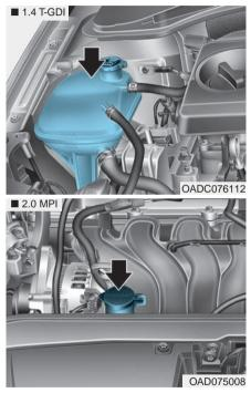
Check the condition and connections of all cooling system hoses and heater hoses. Replace any swollen or deteriorated hoses. The coolant level should be filled between the F and the L marks on the side of the coolant reservoir when the engine is cool.
