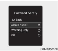
• The driver can activate the FCA by placing the ignition switch to the ON position and by selecting:
