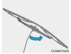
1. Raise the wiper arm and slightly rotate the wiper blade assembly to expose the plastic locking clip.
