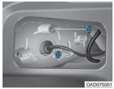
Loosen the assembly retaining nuts.
