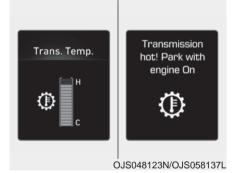
• Select trip computer mode on the LCD display and move to the transmission temperature screen to see the temperature of the dual clutch transmission.
