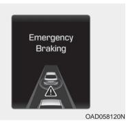
This warning message appears on the LCD display with a warning chime.
