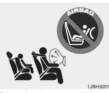
Even though your vehicle is equipped with the OCS, never install a child restraint in the front passenger's seat. An inflating air bag can forcefully strike a child or child restraint resulting in serious or fatal injury.
