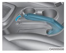
Always set the parking brake before leaving the vehicle. To apply the parking brake:
