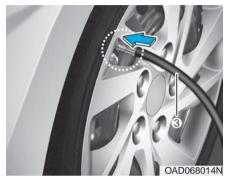
4. Unscrew the valve cap from the valve of the detective wheel and screw the filling hose (3) of the sealant bottle onto the valve.
