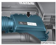
The air cleaner filter can be cleaned for inspection using compressed air.
