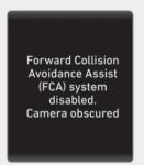
However, the FCA may not properly operate in an area (e.g. open terrain), where any substances are not detected or the camera is blocked with dirt, snow or debris after turning ON the engine.
