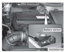
The battery sensor is deactivated, when the battery is disconnected from the negative pole for maintenance purpose.
