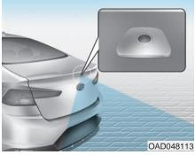
The Rear View Monitor will activate when the engine is running and the shift lever is in the R (Reverse) position. This is a supplemental system that provides a view of the area behind the vehicle through the display audio or AVN screen while the vehicle is in the R (Reverse) position.
