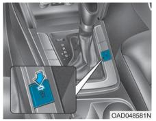
The ISG OFF button indicator illuminates. Auto Stop is Off. Start vehicle manually
