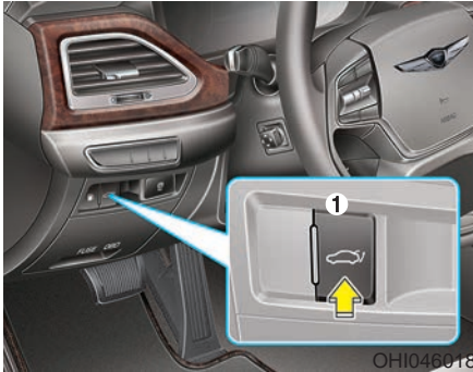
(2) Power Trunk Open button
