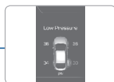
Low Tire Pressure / Tire Pressure Monitor / TPMS Malfunction Display (shown on the cluster LCD display)
