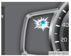
8. Check if the charging indicator light of the high voltage battery in the instrument cluster is turned ON. Charging is not done when the charging indicator lamp is OFF.
