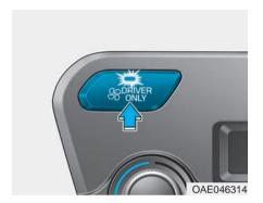
If you press the DRIVER ONLY button(\$\mathbf{s}^{DRIVER}\_{ONLY}) and the indicator light illuminates, cold air mostly blows in the direction of the driver's seat. However, some of the cold air may come out of other seating position ducts to keep indoor air pleasant.
