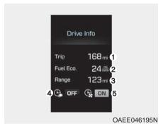
At the end of each driving cycle, the Driving Info message is displayed. This display shows the trip distance (1), average fuel economy (2), remaining vehicle range (3), charging time status (4) and climate time status (5).
