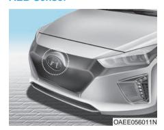
In order for the AEB system to operate properly, always make sure the radar sensor cover is clean and free of dirt, snow, and debris. Dirt, snow, or foreign substances on the lens may adversely affect the sensing performance of the sensor.
