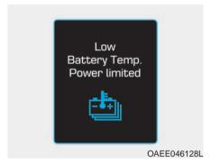
This warning message is displayed to protect battery and electric vehicle system when the high voltage battery temperature is too low.
