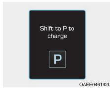
This message is displayed if you connect the charging cable without the gear in the P (Park) position.
