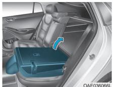
7. To use the rear seat, lift and unfold the seatback to the upright position. Push the seatback firmly until it clicks into place. Make sure the seatback is locked in place.
