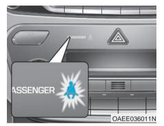
As a reminder to the front passenger, the front passenger's seat belt warning lights will illuminate for approximately 6 seconds each time you turn the POWER button to the ON position regardless of belt fastening.
