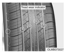
If the tire is worn evenly, a tread wear indicator will appear as a solid band across the tread. This shows there is less than 1/16 inch (1.6 mm) of tread left on the tire. Replace the tire when this happens.
