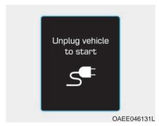
This message is displayed when you start the vehicle without unplugging the charging cable. Unplug the charging cable, and then start the vehicle.
