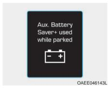
This message is displayed when the Aux. Battery Saver+ function has been completed.
