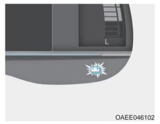
When there are 2~3 gauge bars (near the "L (Low)" area) on the SOC gauge, the warning lamp turns ON to alert you of the battery level.
