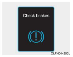
This warning message is displayed when the brake performance is low or the regenerative brake does not work properly due to a failure in the brake system.
