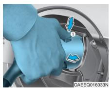
Hold the charging connector handle and pull it while pressing the release button (1).
