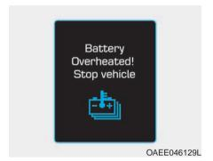
This warning message is displayed to protect battery and electric vehicle system when the high voltage battery temperature is too high.
