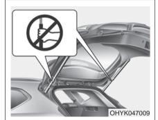
Do not hold the part (gas lifter) that supports the liftgate. Be aware that the deformation of the part may cause vehicle damage and a risk of safety accident.
