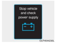
This warning message is displayed when a failure occurs in the power supply system.
