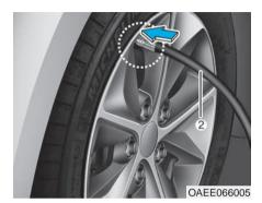
5. Unscrew the valve cap from the valve of the flat tire and screw the filling hose (2) of the sealant bottle onto the valve.
