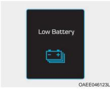
When the high voltage battery level reaches below 13%, this warning message is displayed.
