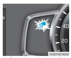
11. Check if the charging indicator light of the high voltage battery in the instrument cluster is turned ON. Charging is not done when the charging indicator lamp is OFF.
