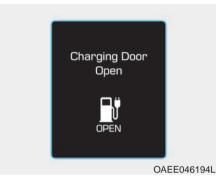
This message is displayed when the vehicle is driven with the charging door opened. Close the charging door and then start driving.
