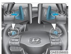
The paddle shifter is used to adjust the regenerative braking rate from 0 to 3 during decelerating or braking.
