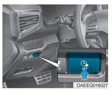
If you press the scheduled charging deactivation (((Spt))) button to immediately charge the battery, charging must be initiated 3 minutes after the charging cable has been connected.
