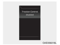
Press the ESC OFF button briefly. The ESC OFF indicator light and message "Traction Control disabled" will illuminate. In this state, the traction control function of ESC is disabled, but the brake control function of ESC still operates.
