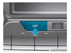
Push the OFF button to turn the climate control system off. You can still operate the mode and air intake buttons as long as the POWER button is in the ON position.
