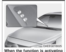
the third Charging Indicator Lamp will blink and high voltage electricity will be flowing in the vehicle. Do not touch the high voltage electric wire (orange), connector, and all electric components and devices. This may cause electric shock and lead to injuries. Also, do not modify your vehicle in any way. This may affect your vehicle per-
