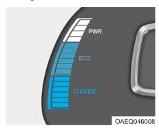
The ECO guide shows the energy consumption rate of the vehicle and the charge/discharge status of the regenerative brakes.
