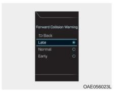
The driver can select the initial warning activation time on the LCD display. Go to the 'User Settings  $\rightarrow$  Driving
