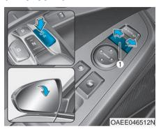
When you shift the vehicle to R (Reverse) position, the side view mirror(s) will rotate downwards to aid with driving in reverse. The position of the side view mirror switch (1) determines whether or not the mirrors will move:
