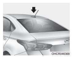
The roof antenna receives AM/FM signals.
