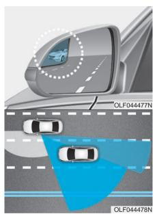
The Blind Spot Mirror (BSM) is a supplemental mirror that helps reduce the driver's blind spot by showing the rear side area of the vehicle. The blind spot mirror is equipped on the left-hand side view mirror.
