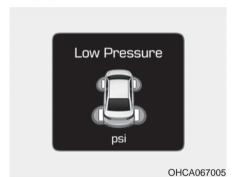
system warning indicators are illuminated and the warning message is displayed on the cluster LCD display, one or more of your tires is significantly under-inflated. The LCD position indicator will indicate which tire is significantly under-inflated by illu-
