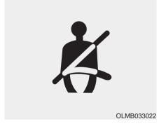
As a reminder to the driver, the seat belt warning light will illuminate for approximately 6 seconds each time you place the ignition switch to the ON position regardless of belt fastening. However, if the seat belt is unfasted, a warning chime will sound for approximately 6 seconds.
