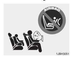
Even though your vehicle is equipped with the OCS, never install a child restraint in the front passenger's seat. An inflating air bag can forcefully strike a child or child restraint resulting in serious or fatal injury.
