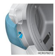
Remove the rear combination lamp assembly from the body of the vehicle.
