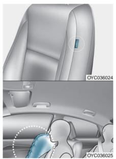
Your vehicle is equipped with a side air bag in each front seat. The purpose of the air bag is to provide the vehicle's driver and the front passenger with additional protection than that offered by the seat belt alone. The side air bags are designed to deploy only during certain side impact collisions, depending on the crash severity.
