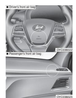
The purpose of the SRS is to provide the vehicle's driver and front passengers with additional protection than that offered by the seat belt system alone. The advanced SRS offers the ability to control the air bag inflation within two levels. A first stage level is provided for moderate-severity impacts.
