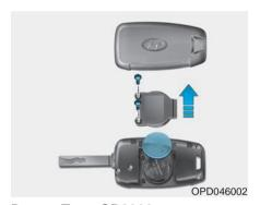
Battery Type: CR2032 To replace the battery:
