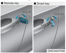
If you lock the driver's door with a mechanical key, all vehicle doors will lock. If you unlock the driver's door with a mechanical key, the driver's door will unlock and the passenger doors will unlock according to the current two press unlock setting.
