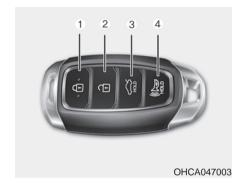
Your HYUNDAI uses a Smart Key, which you can use to lock or unlock a door (and trunk) and start the engine.
