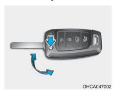
If the remote key does not operate normally, you can lock or unlock the driver's door by using the mechanical key.
