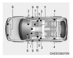
The SRS consists of the following components:
