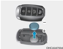
If the Smart Kev is not working properly. try replacing the battery with a new one. Battery Type: CR2032
