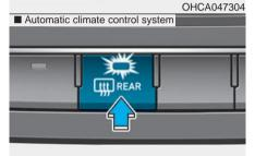
The defroster heats the window to remove frost, fog and thin ice from the interior and exterior of the rear window, while the engine is running.
