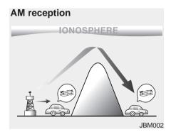
AM broadcasts can be received at greater distances than FM broadcasts. This is because AM radio waves are transmitted at low frequencies. These long distance, low frequency radio waves can follow the curvature of the earth rather than travelling straight. In addition, they curve around obstructions resulting
