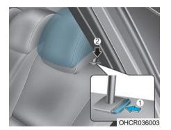
2. Lower the rear head restraints to the lowest position by pushing and holding the release button (1) and pushing down on the headrest (2).
