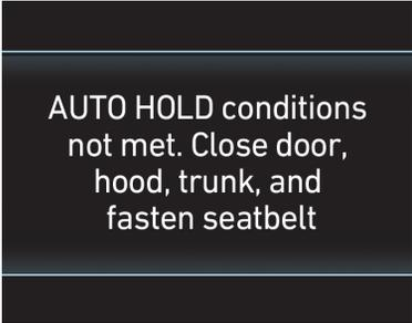
AUTO HOLD conditions not met. Close door, hood, trunk, and fasten seatbelt
