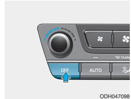
Push the OFF button of the front to turn off the air climate control system. However, you can still operate the mode and air intake buttons as long as the Engine Start/Stop button is in the ON position.
