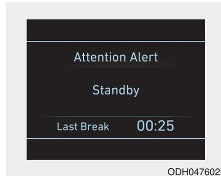
The Driver Attention Alert system enters the ready status and displays the 'Standby' screen in the following situations.
