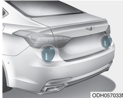
The sensors are located inside of the rear bumper.
