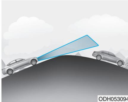
During uphill or downhill driving, the Smart Cruise Control System may not detect a moving vehicle in your lane, and cause your vehicle to accelerate to the set speed. Also, the vehicle speed will rapidly decrease when the vehicle ahead is recognized suddenly.
