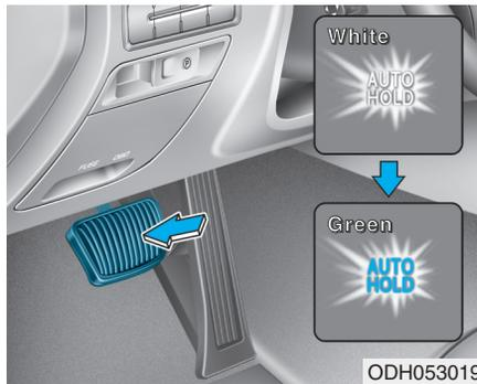
2. When you stop the vehicle completely by depressing the brake pedal, the Auto Hold maintains the brake pressure to hold the vehicle stationary. The indicator changes from white to green.
