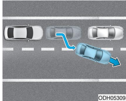
When driving in stop-and-go traffic, and a stopped vehicle in front of you merges out of the lane, the AEB system may not immediately detect the new vehicle that is now in front of you. In this case, you must maintain a safe braking distance, and if necessary, depress the brake pedal to reduce your driving speed in order to maintain a safe distance.
