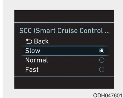
The sensitivity of vehicle speed when following the front vehicle to maintain the set distance can be adjusted. Go to the 'User Settings → Driving Assist → SCC (Smart Cruise Control Response) → Slow/Normal/Fast' on the LCD display. You may select one of the three stages you prefer.
