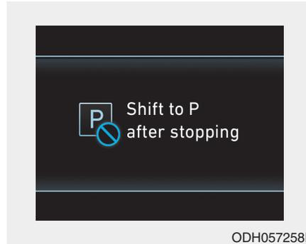
The warning message appears on the LCD display, when the brake pedal is not depressed while shifting the gear.
