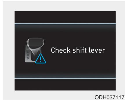
The warning message appears on the LCD display, when there is a malfunction with one of the key transmission shifter components. In this case, we recommend you to immediately have the vehicle inspected by an authorized retailer of Genesis Branded products.
