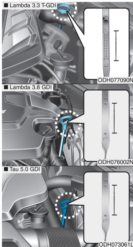
6. Pull the dipstick out again and check the level. The level should be between F and L.
