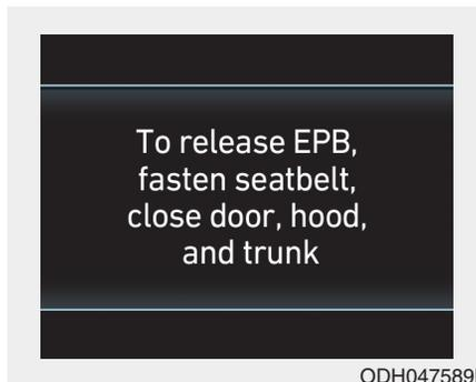
To release EPB, fasten seatbelt, close door, hood, and trunk
