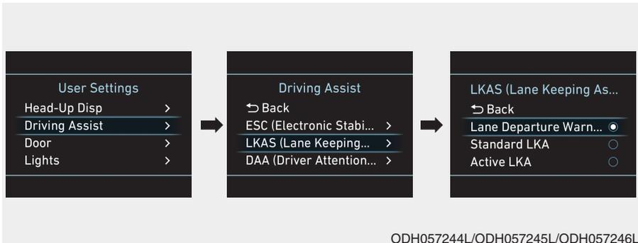
The driver can change LKAS to Lane Departure Warning System (LDWS) or the LKAS mode between Standard LKA and Active LKA from the User Settings Mode on the LCD display.
