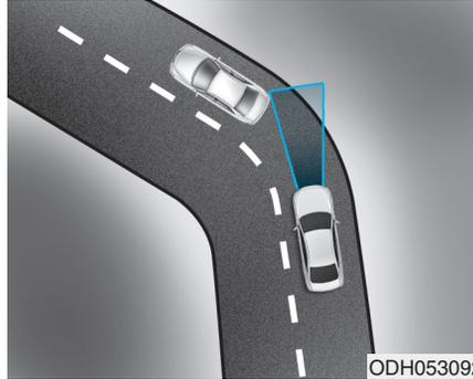
The Smart Cruise Control System may not detect a moving vehicle in your lane, and then your vehicle could accelerate to the set speed. Also, the vehicle speed will decrease when the vehicle ahead is recognized suddenly.
