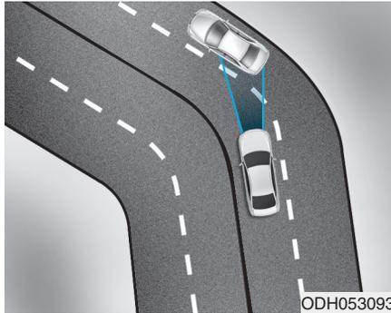
The AEB system may recognize a vehicle in the next lane when driving on a curved road.
