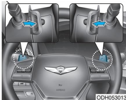
The paddle shifter is available when the shift lever is in the D (Drive) position or the manual shift mode.
