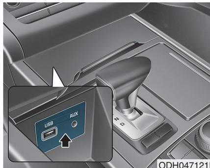
You can use an AUX port to connect audio devices and an USB port to plug in an USB and also in an iPod® port.
