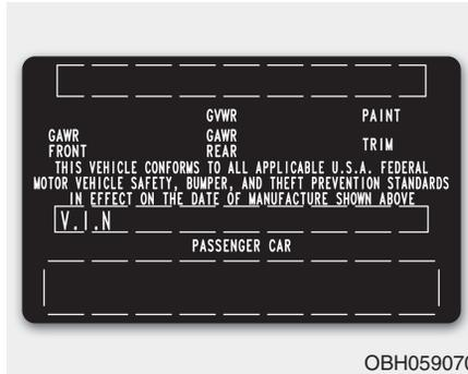
The certification label is located on the driver's door sill at the center pillar and shows the maximum allowable weight of the fully loaded vehicle. This is called the GVWR (Gross Vehicle Weight Rating). The GVWR includes the weight of the vehicle, all occupants, fuel and cargo.
