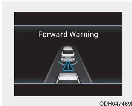
This initial warning message appears on the LCD display and the head up display (if equipped) with a warning chime.
