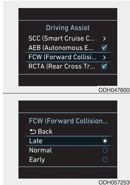
The driver can select the initial warning activation time in the User Settings in the LCD display.
