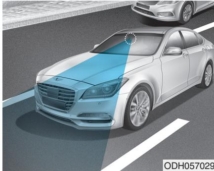
The Lane Keeping Assist System detects the lane markers on the road with a camera at the front windshield, and assists the driver's steering to help keep the vehicle in the lanes.
