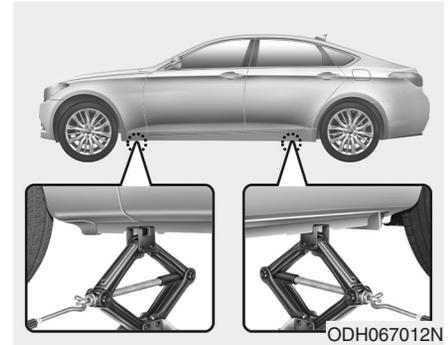
8. Place the jack at the designated jacking position under the frame closest to the tire you are changing. The jacking positions are plates welded to the frame with two tabs and a raised dot. Never jack any other position or part of the vehicle. It may damage to the side seal molding.
