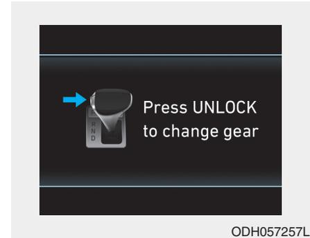
The warning message appears on the LCD display, when the [UNLOCK] button is not pressed while shifting the gear. We recommend you press the [UNLOCK] button and then shift the gear.
