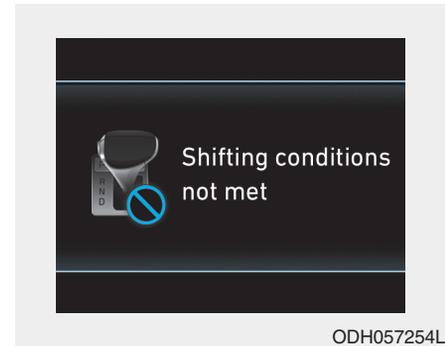
The warning message appears on the LCD display, when engine RPM is too high, or when driving speed is too fast to shift the gear. We recommend you decrease the engine speed or slow down before shifting the gear.
