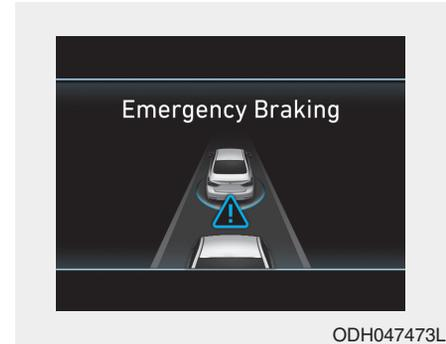
This warning message appears on the LCD display and the head up display (if equipped) with a warning chime.
