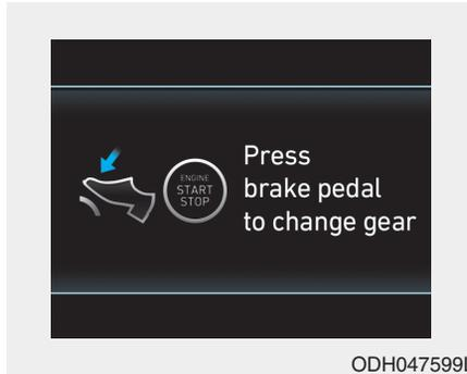
The warning message appears on the LCD display, when the brake pedal is not depressed while shifting the gear.
