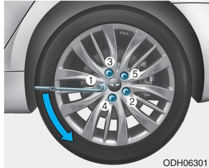
7. Loosen the wheel lug nuts counterclockwise one turn each in the order shown above, but do not remove any lug nuts until the tire has been raised off of the ground.
